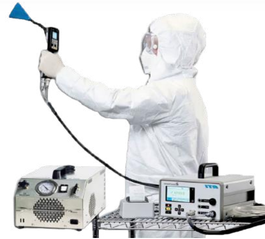
HEPA Filters Integrity Test
